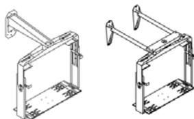
Available in a range of sizes and featuring easy adjustment in both height and width, the Jumbo 2000 will provide a secure mount for almost any monitor up to 42" (106 cm), including those with wide screen aspect ratio. Also, optional security fasteners (ACC 502) are available to make the Jumbo 2000 tamper-resistant. An optional VCR bracket is available and can be added at any time, even after the monitor is already in place.
