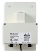
Where in-room power supplies are needed and new wall brackets are to be used, the built-in power supply wall bracket offers a neater, less expensive means of installing individual TV power supplies. These units feature fuse protected primary and secondary circuits and are equipped with 6-foot power cords with hospital grade plugs. Each has a 75 Ohm TV signal input connector.
