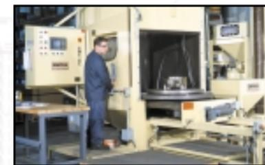
Computerized Empire Abrasives Shot Peening Machine increases strength and durability of the metal parts.
